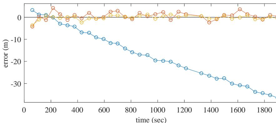
**Fig. 3.** Position error at the marker points relative to the marker tags in the reference ride. The blue curve shows the recorded distance of the speed sensor, the red curve the distance determined by projecting the GPS coordinate onto the reference trajectory and the yellow curve shows the result of the Kalman filtering.
