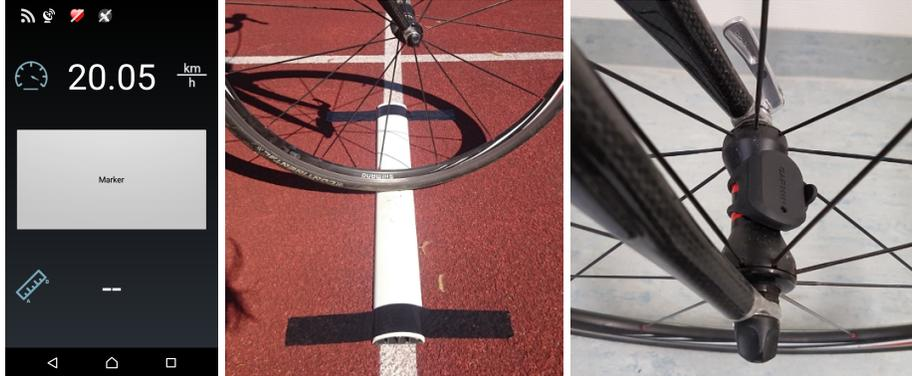
**Fig. 2.** Experimental setup: The left picture shows a screenshot of the application. The number in the top shows the current speed and the gray box is the button that was pressed each time the marker was passed. The picture in the middle shows the physical realization of the marker: A rounded bar, taped on the 50m line of the track. The Garmin hub speed sensor is presented in the right picture, mounted on the hub of the front wheel of the test bike.
