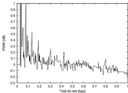
**Fig. 5.** JPEG 2000: Difference in expected PSNR between progressive optimal EPS and an optimal 1 bpp EPS for BER 0.1. For clarity, the PSNR axis was truncated at 1 dB.
