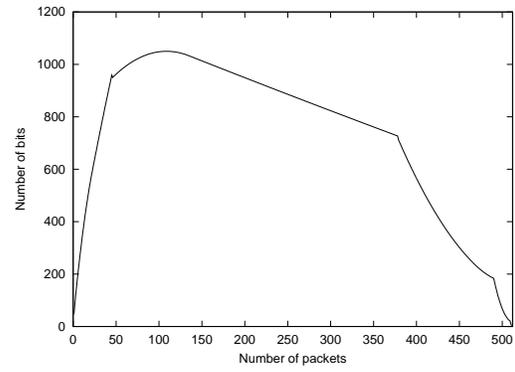
**Fig. 1.** Difference in the expected number of received source bits as a function of the number  $n$  of packets sent between  $n$ -packet optimal EPS and an EPS that is optimal for target rate 1.0 bpp. The BER was equal to 0.1.
