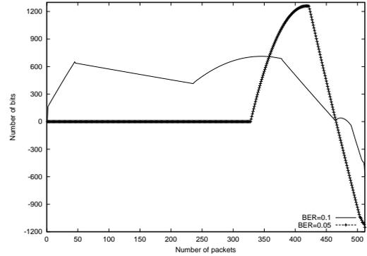
**Fig. 2.** Difference in the expected number of received SPIHT source bits between progressive optimal EPS and an optimal 1 bpp (512-packet) EPS for BER 0.05 and 0.1.
