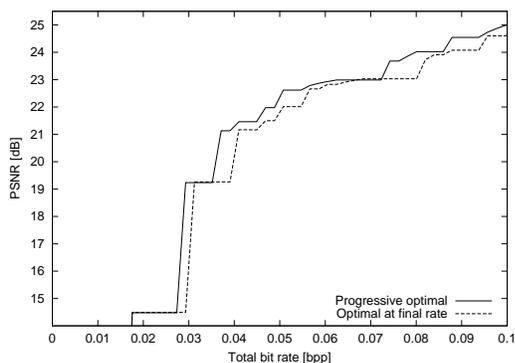
**Fig. 6.** JPEG 2000: Expected PSNR between progressive optimal EPS and an optimal 1 bpp EPS for BER 0.1.
