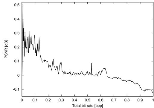
**Fig. 3.** Difference in expected PSNR between progressive optimal EPS and an optimal 1 bpp EPS for BER 0.1.
