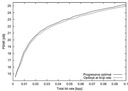
**Fig. 4.** Expected PSNR for progressive optimal EPS and an optimal 1 bpp EPS for BER 0.1. Results are shown up to total rate 0.1 bpp.
