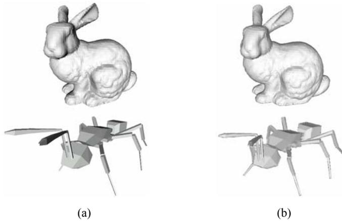
Figure 3. Result of the surfelization: the original triangulated models (a) and the corresponding surfel-based representations (b).
