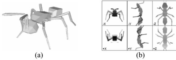
Figure 2. Surfel-based model (a) and the extracted depth buffer images (b).
