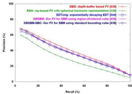
Figure 4. Precision-recall diagram computed for different feature vectors of the original triangles meshes with respect the proposed feature vector extracted from the corresponding surfel-based models. Dimension of feature vectors are given in brackets.
