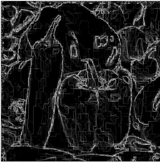
Figure 3: Gradient image of reconstructed Peppers 512x512, compression ratio 76:1, adaptive split-and-merge partition, block size 8, 800 ranges, threshold 10.
