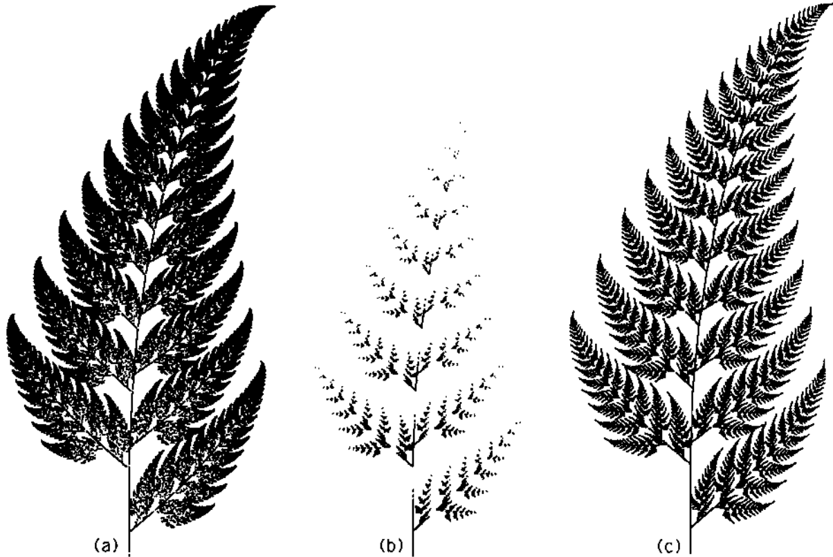
Figure 6: A comparison of three attracting methods for the rendering of the set generated by an IFS. (a) The stochastic method using N_1 = 198,541 points. The probabilities used in the method are 0.01, 0.07, 0.07 and 0.85 corresponding to the four transformations given in the Appendix. (b) Evaluation of the tree of transformations to a given depth n = 9 , resulting in N_2 = 349,525 points (often overlapping on the grid). (c) The adaptive-cut algorithm using N_3 = N_1 points.
