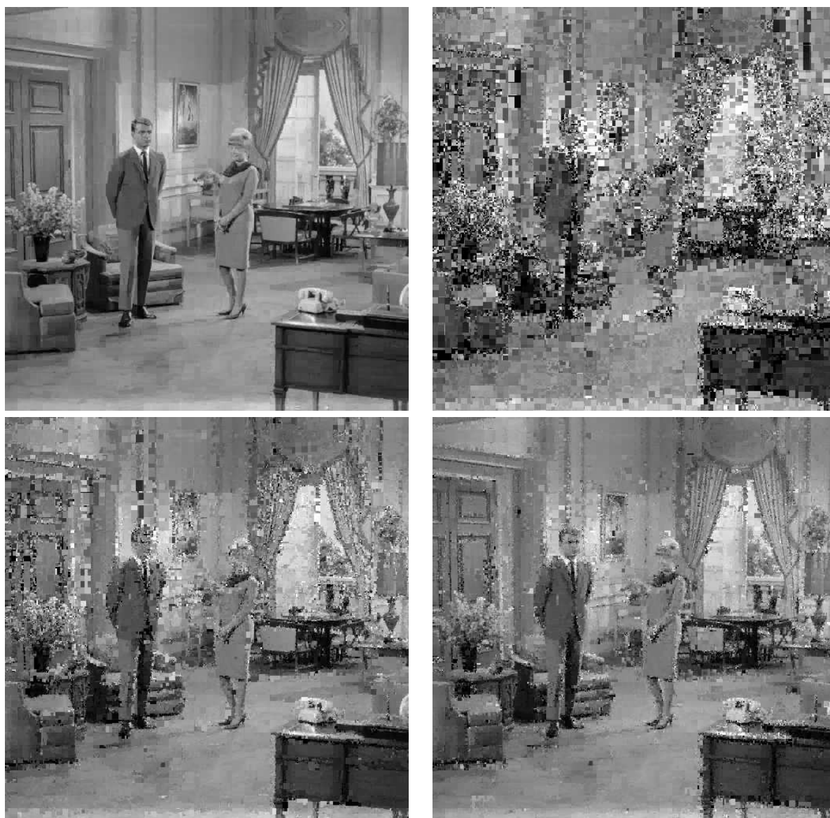
Fig. 7. The fixed point image (upper left), and the second iterate with respectively the conventional decoding (upper right), the proposed method with the natural ordering (lower left), and the proposed method with the ordering based on range frequencies (lower right). The partition consists of 4879 ranges, 190 of which with zero frequency.
