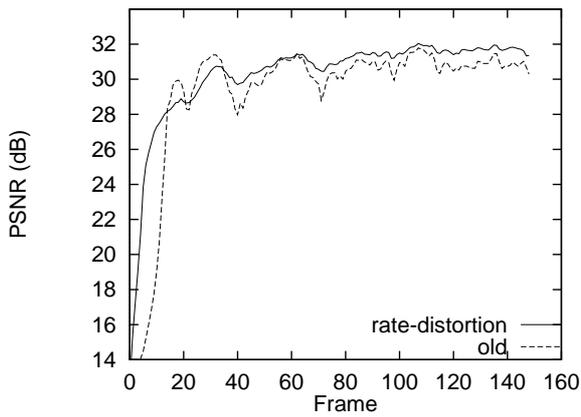
Figure 1: Frame course of PSNR for Y component of the Salesman sequence at 0.137 bpp.
