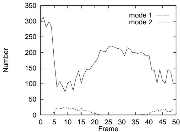
Figure 3: Statistics on the mode in which source vectors are encoded in the Miss America sequence coded at 0.137 bpp.
