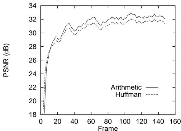
Figure 7: Comparison between Huffman coding and adaptive arithmetic coding for the rate-distortion coder for the Salesman sequence at 0.137 bpp.
