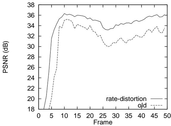
Figure 2: Frame course of PSNR for Y component of the Miss America sequence at 0.137 bpp.
