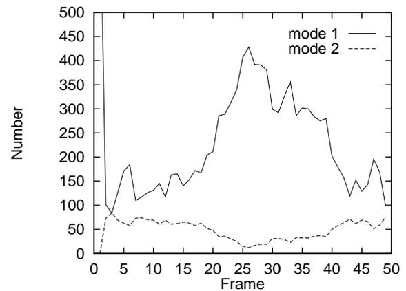
Figure 6: Statistics on the mode in which source vectors are encoded in the Miss America sequence coded at 0.312 bpp.
