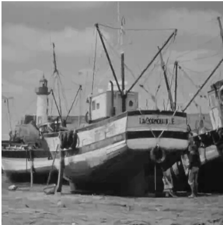
Figure 4: The 512 \times 512 Boat image coded with OMSGVQ at 0.25 bpp and post-processed with the technique in [8]. The PSNR is equal to 30.35 dB.
