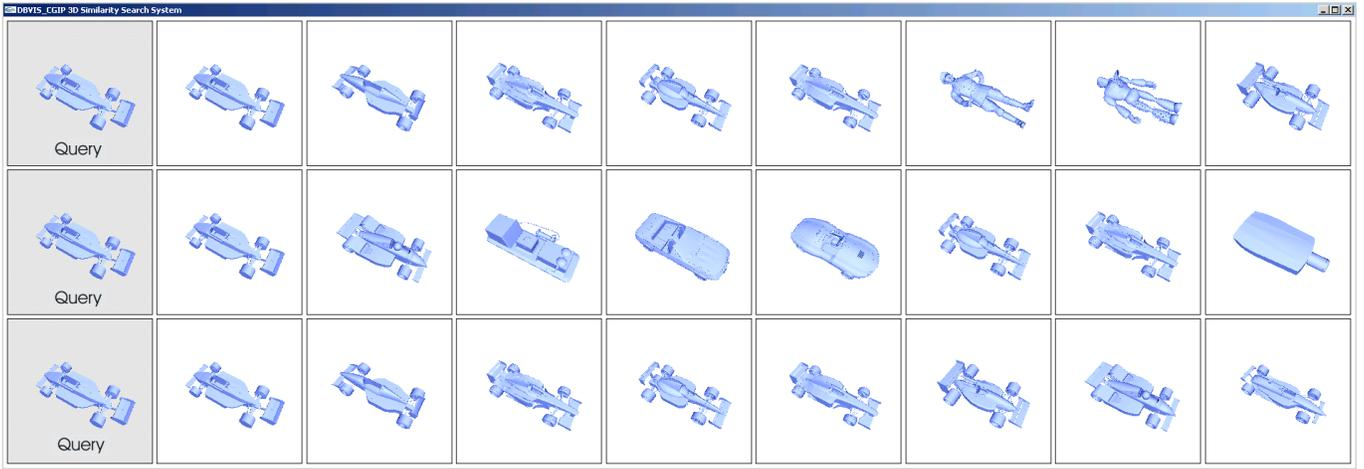
Fig. 1. Example of three similarity queries (with the same query object) using depth buffer, silhouette, and a combination of both descriptors
