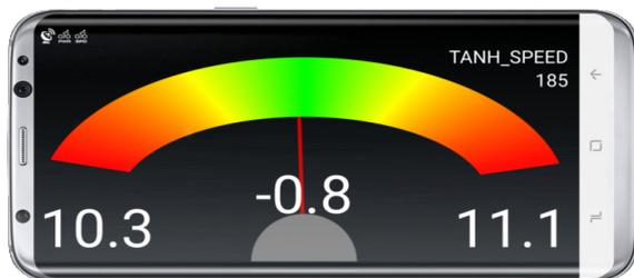
feedback screens had the same base layout with a scale from red to green to red (see figure on the left) Three labels show current measured value, target value and the difference between them.
