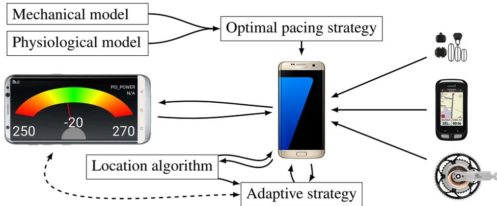
Figure 1: A Galaxy S8 smartphone is chosen as the central component that collects data, adapts the strategy for the current position and exhaustion state and displays the result to the cyclist.
